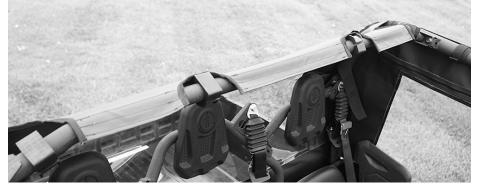
7. The sides of the Rear Window will attach to the Velcro tabs from the doors. The one exception is the top corners that have a double-sided tab that is held in place by a 3" adhesive strip. The bottom of the Rear Window will hang between the bed and the backs of the seats. See photos below.
