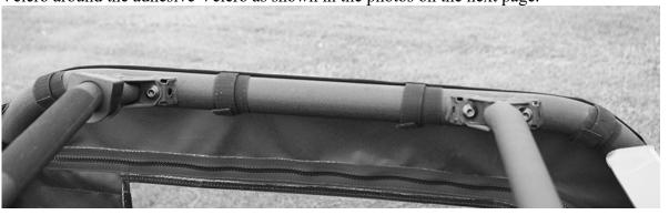
2. The rear edge of the doors has a 3 strips of Velcro sewn down the entire length. Starting at the top use the 6", 16" and 8" adhesive strips to attach the door to the roll cage. This attaches to the Velcro sewn down the sides of the rear window. See photos below.
