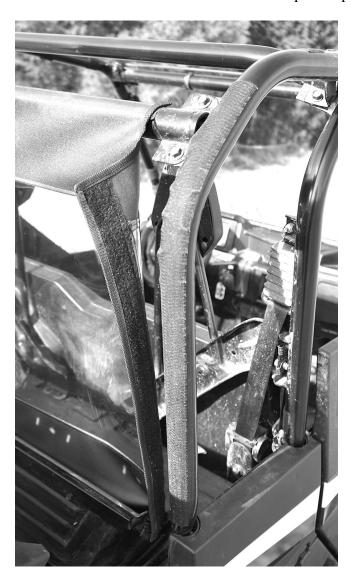
5. Next place two 3" adhesive strip on the center bar towards the bottom to match up with the two tabs as shown in the photo below.
