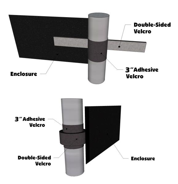
4. Next take the 30" adhesive Velcro strips and run it down the back of the roll cage facing towards the rear of the vehicle. Start at the bottom and work your way up the bar. You will see the double-sided Velcro tabs sewn along the back of the doors that will attach to this strip. See photo below.
