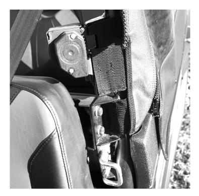
6. Last piece of Velcro is the 3" strip on the end of the front strip as shown in the photo below.
