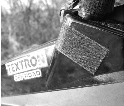
7. Once all the Velcro is in place the last thing to do is install the screw snap studs. NOTE: The best way to install the snap studs is to put them in the sockets in the door first. Then push them into the plastic to make a mark. Then pull the screw stud out and screw it into the plastic where the mark was made. See Photos on next page.
