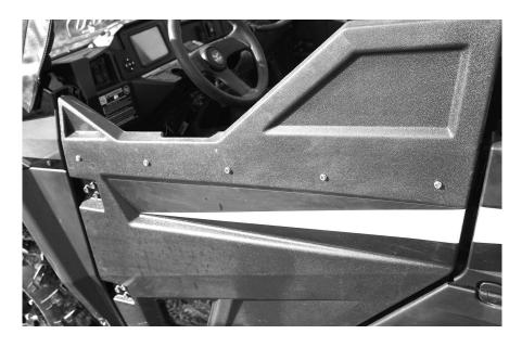
8. Final step on the doors are to install the polycarbonate panel in the hole at the bottom of the factory half door. Take the panel screws and install the panel on the inside of the door as shown in the pictures below.
