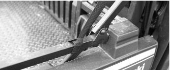
7. Once all the straps are in place run them through the buckles. Pull them tight making sure the top is centered and the side seams line up correctly along the roll cage. The diagram below shows how to lace the webbing through the buckle.
