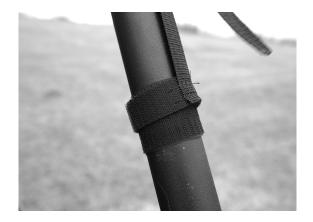
6. The rear of the Top Cap is held in place using the straps that have a loop sewn in one end. Take the end of the strap with the loop and put it under the bed rail just behind the support bar. Then take the other end of the strap and run it through the loop, pulling it tight. The photo below shows what it should look like.
