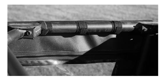
5. The rear edge of the front door also has double-sided strips as well but you do not use the 3" adhesive strips for it. Instead place the 45" adhesive strips down the backside of the middle bar facing the rear of the vehicle. You will need to cut the adhesive strip and place part of it above and below the mount for the bar as shown in the photo. See photo below.
