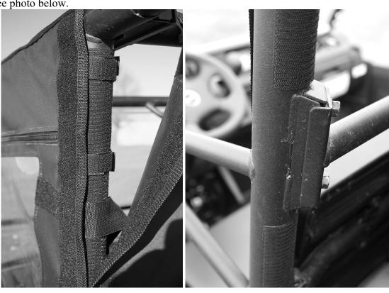
6. The diagrams below show how the double-sided straps and the 3" adhesive Velcro works.
