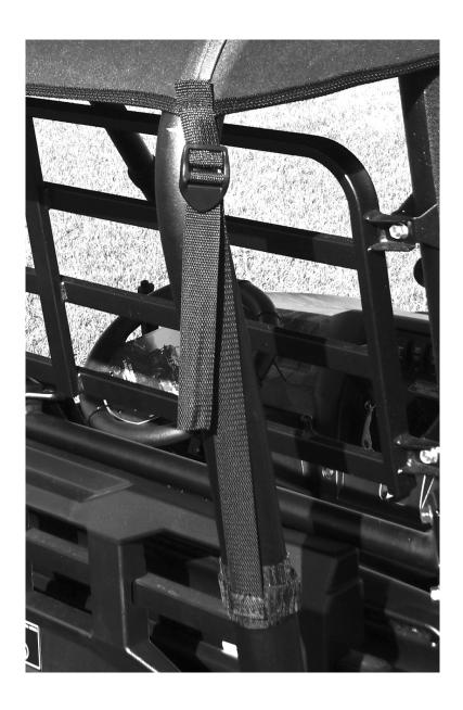
4. Once all the straps are in place run them through the buckles. Pull them tight making sure the top is centered and the side seams line up correctly along the roll cage. The diagram below shows how to lace the webbing through the buckle.
