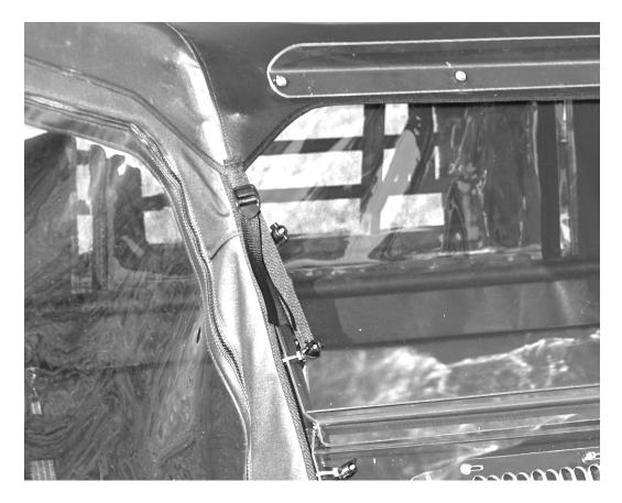
3. The rear of the Top Cap is held in place using the straps that have double-sided Velcro sewn in one end. Take the 6" adhesive Velcro strips and wrap them around the roll cage approximately 12" below the back of the Top Cap. Now take the end of the strap with the Velcro and wrap it around the bar and Velcro as tight as possible. Then take the other end of the strap and run it through the loop, pulling it tight. The photo on the next page shows what it should look like.
