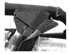
2. Now line the door up with the frame and begin attaching the double-sided Velcro strips as you did with the sides of the Rear Window. Photo below shows where they are.
