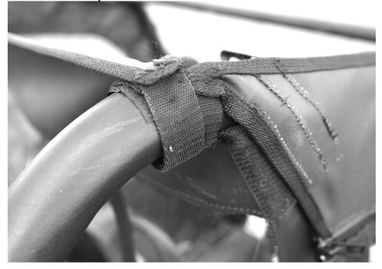
4. Finally, the bottom of the door has Velcro sewn across the entire length. Place the 20" adhesive Velcro strip on the outside of the door to match up with the bottom of the soft door. Also the front corner has a 10" piece of Velcro running vertical. See photo below.
