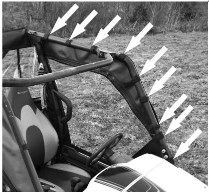
3. After you have the front and top double-sided strips attached you can now attach the strip at the very top rear corner of the door. If you have the Rear Window on it is very likely that the two will be at the same location or right next to each other. This is fine, just wrap one over the other. See photo below.
