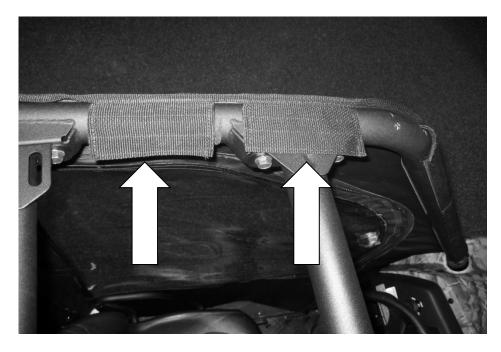
e) Next you will see a 12" Velcro tab running down the rear of the enclosure. Place the matching adhesive Velcro strip on the roll cage and pull the rear window tight side to side. See photo below.
