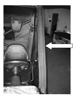
d) Along the top of the doors there are two 5" Velcro loop tabs that should be attached as shown in the photo below. Place the matching adhesive Velcro strips on the roll cage and attach at these points. See photo below.
