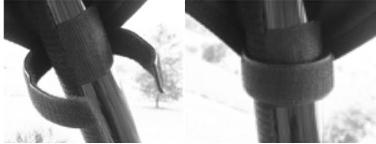
8. Next attach the supplied 10" and 5" adhesive Velcro strips the bottom of the floorboard and the rear of the cab as shown in the photos below.
