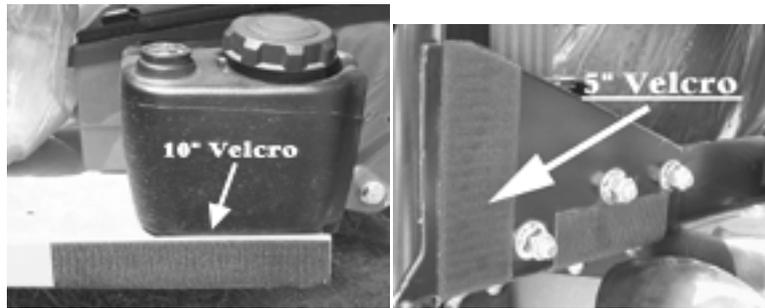
9. The Velcro down the front of the door has a long 30" Velcro tab. If you have a windshield on you Gator you will need to cut the Velcro tab to fit around the mounting hardware. When you cut Velcro tab you must seal the edges with a lighter to prevent fraying.
