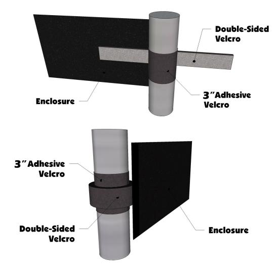
2. Next take the 50" adhesive Velcro strip and run it down the back of the roll cage facing towards the rear of the vehicle. You will see two double-sided Velcro tabs sewn along the back of the doors. The adhesive strip must be aligned so that both tabs can attach to it. See photo below.
