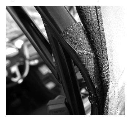
3. Once all the Velcro is in place the last thing to do is install the screw snap studs. NOTE: The best way to install the snap studs is to put them in the sockets in the door first. Then push them into the plastic to make an indention. Then pull the screw stud out and screw it into the plastic where the mark was made. See Photos Below.
