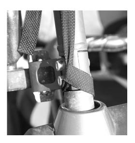
4. Next take the other two straps with a loop sewn on one end and wrap them around the roll cage in the rear just under the safety bar and above the seat belt mount as shown in the photo below.
