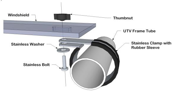
6. Now install the top section of the windshield using the same method as the bottom section with the only difference being that the clamps used for the slanted portion at the top are 1 ½" clamps. Note: The bend at the top of the windshield should be facing toward the rear of the UTV and be placed under the Roll cage at the top. When finished it should look very similar to the diagram below. **Note: Top brace not included in Bush Hog Trail Hunter Windshield.**
