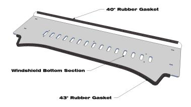
3. Next install the Polycarbonate Vent Slider to the inside face off the bottom section. Begin by removing the protective masking and place the Teflon dots in the corners as shown in the diagram below.
