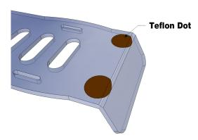
4. Now place the Vent Slider to the Bottom section on the inside face of the windshield as shown in the diagram below. Be sure not to over-tighten the shoulder bolts as this will cause the threaded inserts to spin loose in the Polycarbonate. Just snug those in place with an Allen wrench or finger tight will work.
