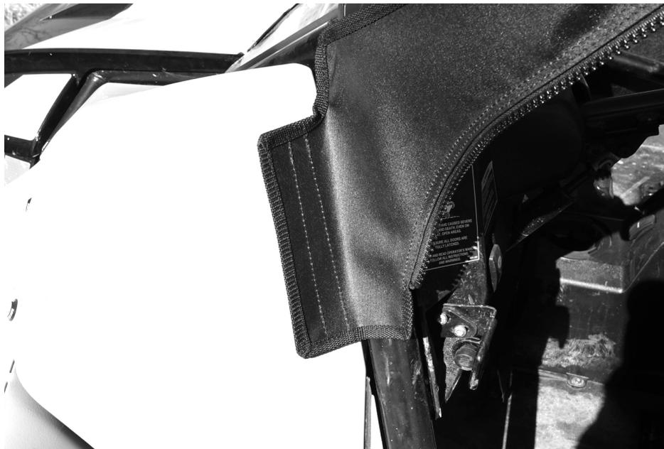
4. Last part of the door to attach is the bottom to the factory half-door. Take the 44” adhesive Velcro strip and attach it to the factory door to match up with the Velcro sewn to the bottom of the soft doors. The adhesive Velcro will cross the hinge of the door, take a knife and cut the adhesive Velcro at the hinge. See the following photos.
