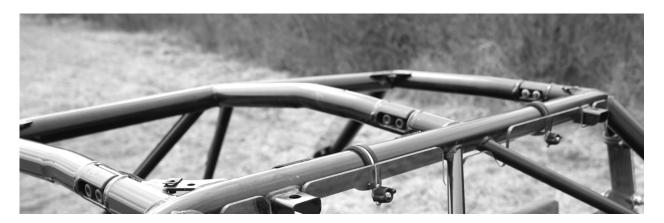
3. Next take the 4 U-Nuts which are black metal clips with a threaded hole and place them in each of the four corners. Each corner has a piece of metal welded in place and has two holes in them. Install the U-Nuts in the smaller of the two holes.
